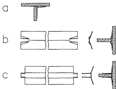
**Figure 7:** Three types of static contact systems used in the SSC resonators.
