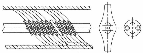
Figure 5: Sliding contact-fingers for the beamline bunchers.
