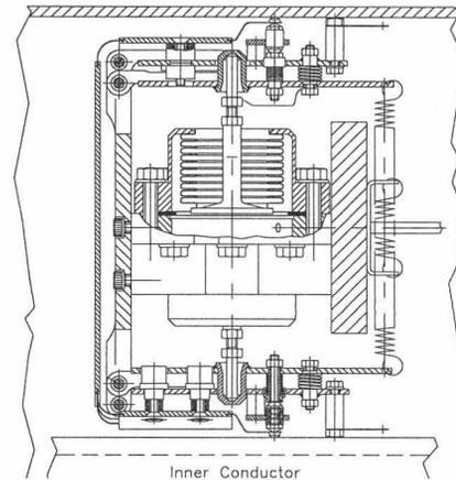
Figure 1: Short-circuiting plate system of the injector resonators.
