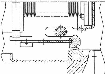
Figure 6: Rolling contact for tuning of the injector resonators.
