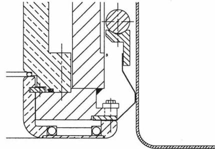
Figure 4: Contact fingers for the SSC capacitors.
