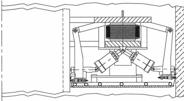
Figure 2: Short-circuiting plate system of the SSC resonators.
