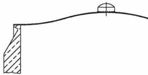
Figure 3: Contact finger of figure 2, showing the profile for welding.
