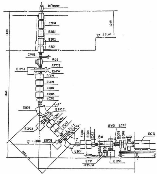
Fig.1 Axial injection line from ECR to SFC
