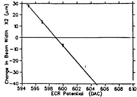
Figure 5: Change in beam width as a function of ECR energy (600=3kV).
