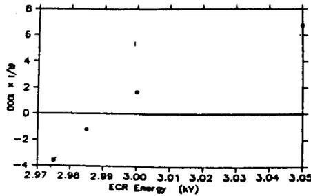
Figure 3: Fractional current change as a function of ECR energy.
