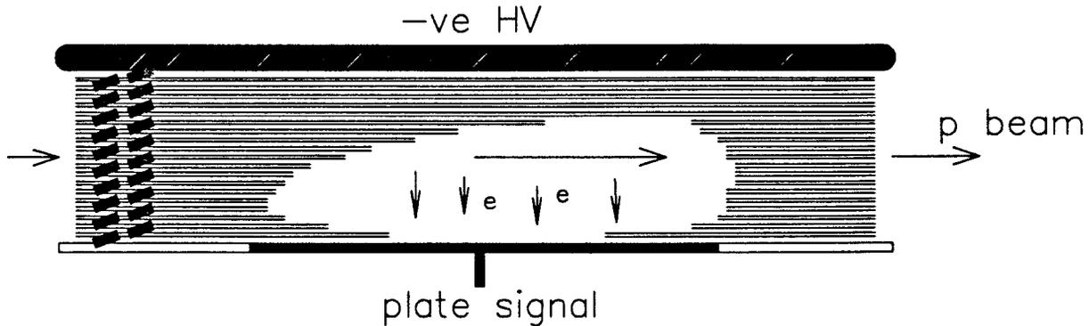
Figure 1: Side view of a transverse field ion chamber. Beam protons ionize the gas; the electrons are collected on the signal plate embedded in the ground plate.
