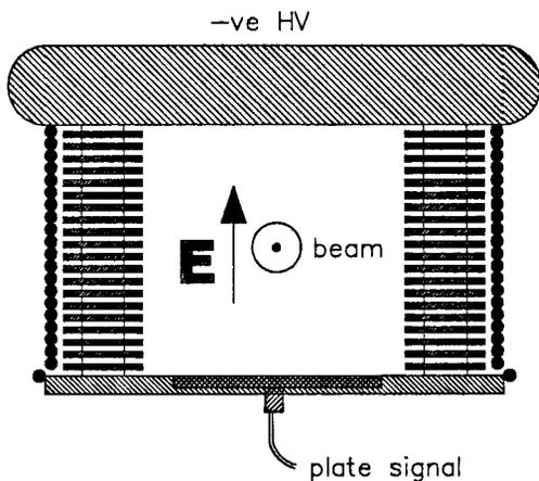
Figure 2: Cross-sectional view through a transverse field ion chamber. Electrodes and ceramic spacers form the side stacks. Resistors across the spacers are mounted on the outside.
