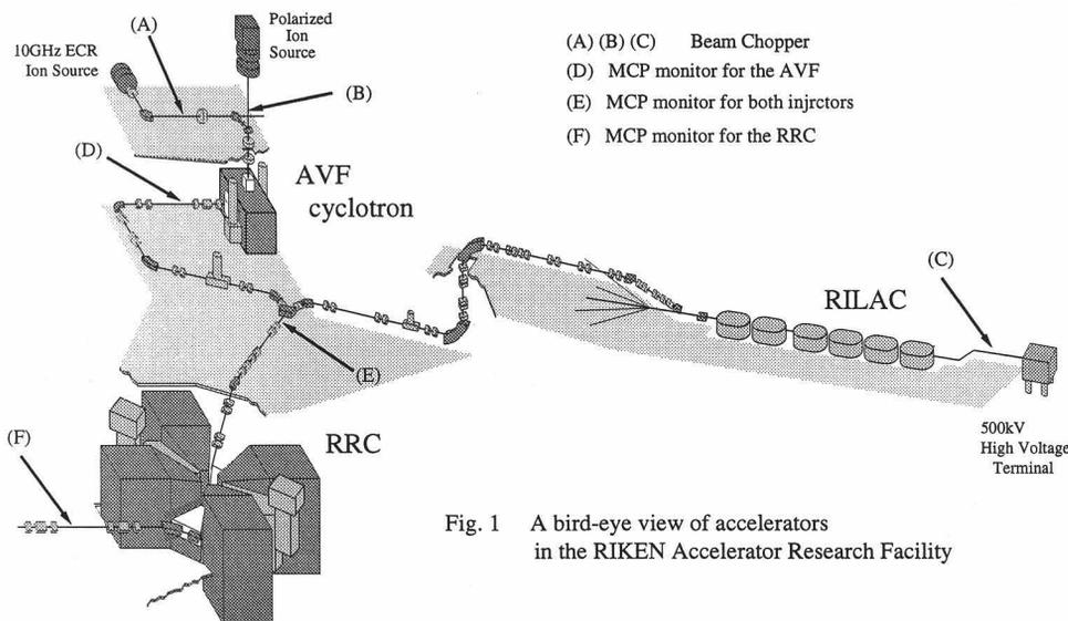
Fig. 1 A bird-eye view of accelerators in the RIKEN Accelerator Research Facility
