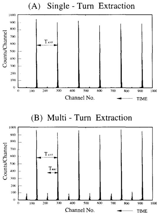
Fig. 5 Time spectra of the extracted beam from the RRC. The beam is 100 MeV/u  $^{18}\text{O}$  and is not chopped. (A) is the case when single turn extraction is realized in more than 99%, and, on the other hand, (B) is when 12% of beam is extracted from the next turn.  $T_{AVF}$  and  $T_{RRC}$  are 68 ns and 34 ns, respectively.
