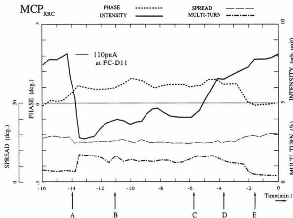
Fig. 6 Example of continuous measurement with the MCP phase probe. Beam intensity (the area of peak in time spectrum), beam phase (peak position), ratio of the multi-turn extraction (shown by a relative fraction of small peaks in Fig. 4 and 5 to the main peaks), and beam bunch spread (peak width in fwhm) are displayed in a duration of 16 min.
