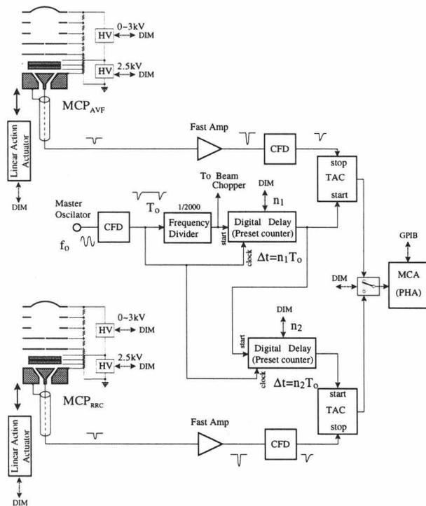
Fig. 3 Block diagram of electronics for the MCP phase monitor. DIM is a remote connection to a host control computer.  $n_1$  and  $n_2$  are the preset values for two digital delay circuits. In the RILAC - RRC operation,  $n_1$  is set one.  $T_0$  is the rf period of the injector.
