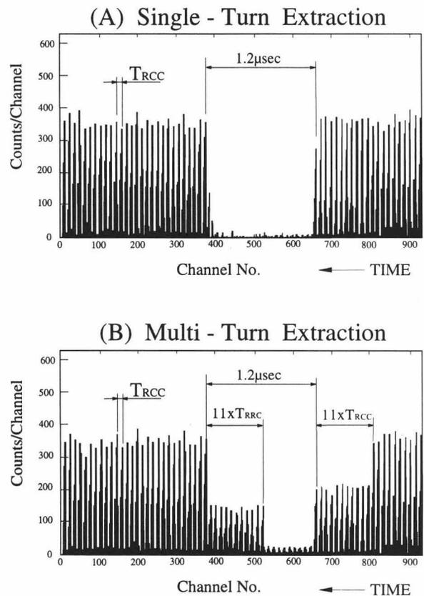
Fig. 4 Time spectrum of the extracted beam from the RRC. The beam is  $^{40}\text{Ar}$  7 MeV/u.  $T_{\text{RCC}}$  is the period of an rf acceleration voltage in the RRC: 56 ns in this case.
