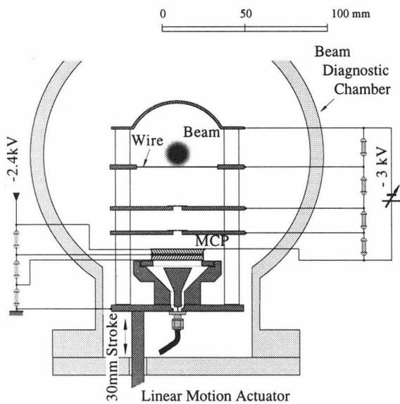
Fig. 2 Cross sectional view of the MCP monitor, which is seen along the beam axis. The MCP is of two-layered type with an available diameter of 14 mm. Double slits in front of the MCP surface prevent the stray electron and/or photons from entering into the MCP.
