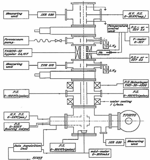
Fig.1. Block schematic of the polarimeter
