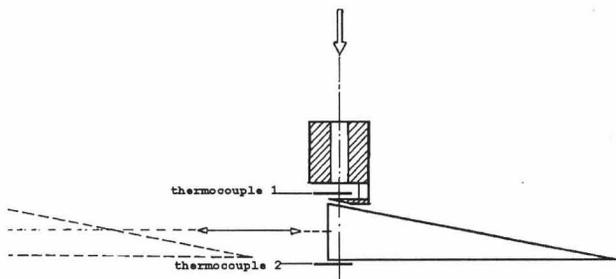
Fig. 4. Principle of the thermal (relative) beam energy measurement device
