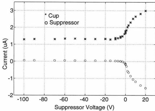
Fig. 6. Cup and biased suppressor currents, N<sup>+</sup> ions.
