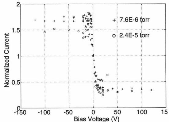
Fig. 4. Current from a biased stainless steel plate, 12 keV N<sup>+</sup> incident beam.
