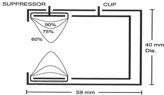
Fig. 5. CERN-ISOLDE style wide aperture Faraday Cup (courtesy E. Kugler) with equipotentials as a percentage of the suppressor bias voltage.
