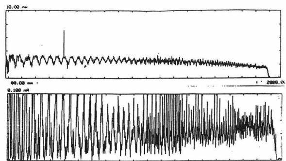
Fig.7. Beam current and turn pattern from the injection to the extraction. Nearly the full transmission is obtained.
