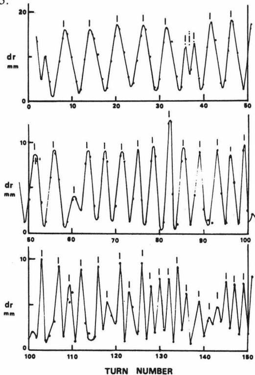
Fig.4. Measured dr separation in each acceleration turn
