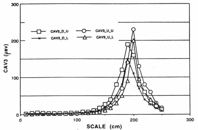
Fig.6. The residual activities measured at cavity-3. The positions shown in this figure are indicated in Figure 2;the first D and U mean the downstream or upstream , the second U and L are for the upper and lower electrodes. The scale should be shortened to the ratio of 1.7/2.0.
