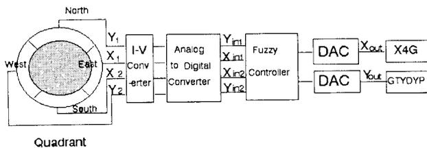
Figure 1: Fuzzy controller for the beam line
