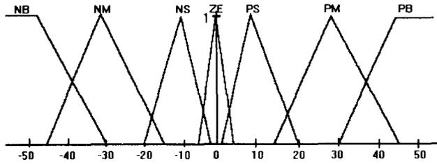
Figure 3: Membership Function of X and Y Axis
