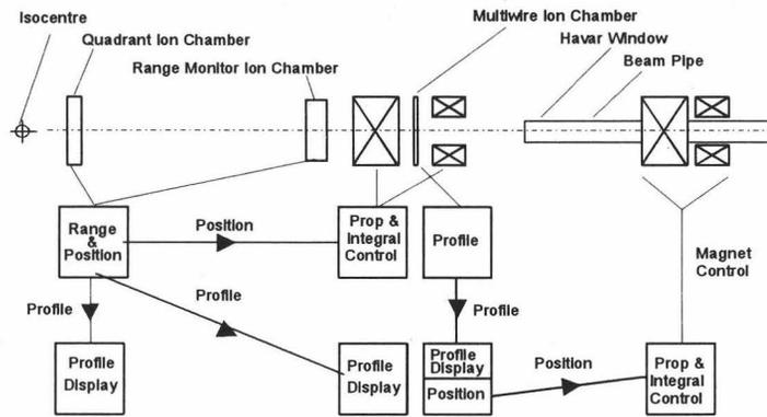
Figure 3. Schematic of the proton therapy beam control system.
