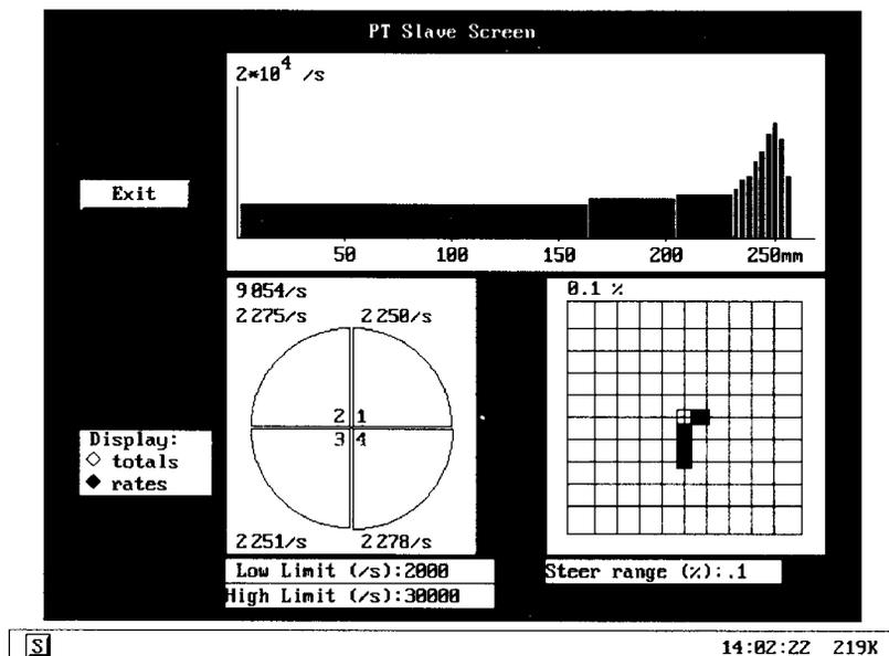
**Figure 2.** Slave screen display showing count rates for the range monitor ionisation chamber (top), the quadrant ionisation chamber (lower left), and the steering signals derived from quadrant count rates (lower right).
