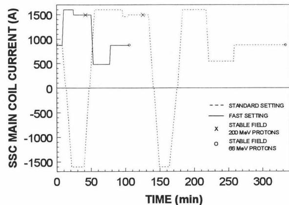
Figure 1. The new fast excitation setting of the sector magnets for isochronous field transitions from 66 to 200 MeV protons and back, compared with the equivalent standard setting method.
