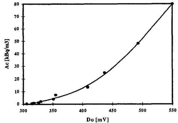
Figure 2b: Calibration curve of the 123-Iodine detector showing the output voltage Do from the SCA2 with the corresponding activity concentration Ac in the detector volume (250ml). The data points are fitted with the 4th order polynomial:  $y = -2.40 \times 10^{-8} x^4 + 4.28 \times 10^{-5} x^3 - 2.60 \times 10^{-2} x^2 + 6.92 \times 10^0 x - 6.80 \times 10^2$ .
