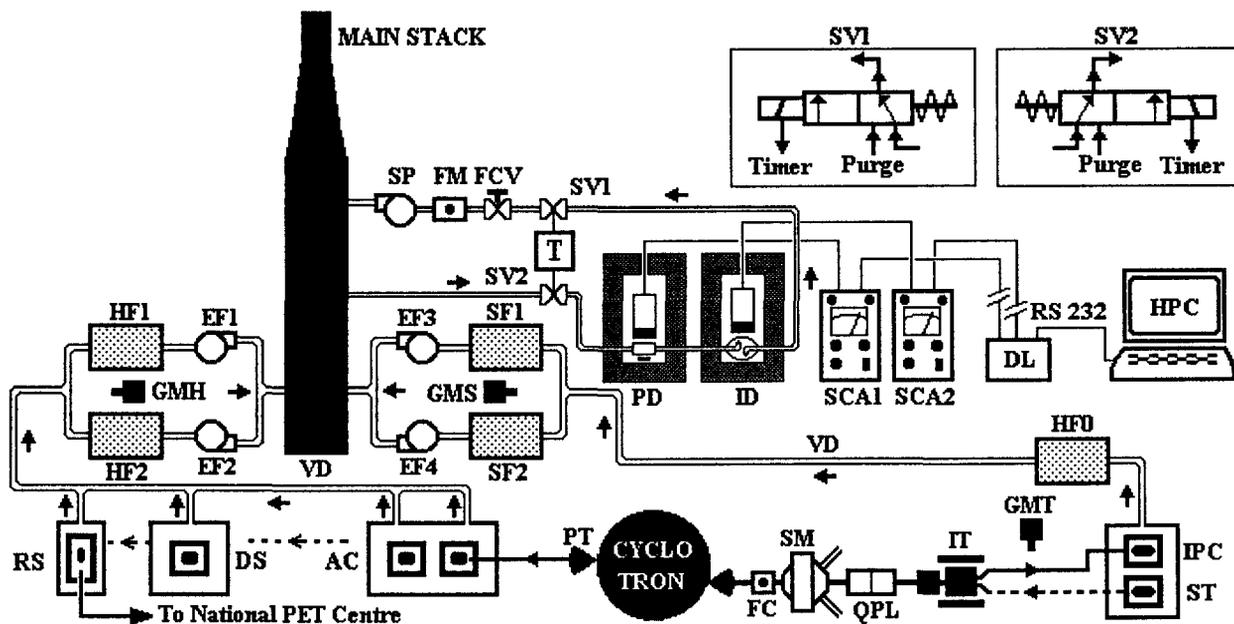
Figure 1: Schematic diagram of the NMC Stack monitoring facility showing the cyclotron targets, hot cells and filter ventilation system, flow control solenoid valves and the real time radiation monitors with the data acquisition system. The diagram is explained in the text.
