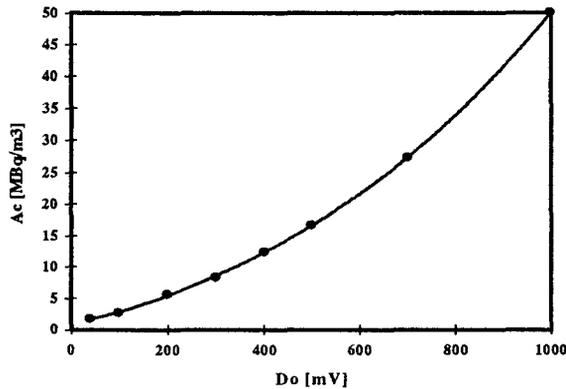
Figure 2a: Calibration curve of the positron detector showing the output voltage Do from the SCA1 with the corresponding activity concentration Ac in the detector volume (3ml). The data points are fitted with the 4th order polynomial:  $y = 1.16 \times 10^{-11} x^4 - 1.33 \times 10^{-8} x^3 + 3.49 \times 10^{-5} x^2 + 1.59 \times 10^{-2} x + 9.19 \times 10^{-1}$ .
