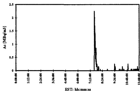
Figure 3a: The results of a typical real time stack discharge analysis during the production of  $^{18}\text{F}$ FDG at the NMC. The back ground noise has been subtracted from the raw data. The instantaneous characteristics of the effluent release is distinctly visible in this figure.
