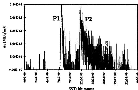
Figure 3b: The results of a typical real time stack discharge analysis during the production of  $^{123}\text{I}$  at the NMC. The back ground noise have been subtracted from the raw data. The instantaneous characteristics of the effluent release is distinctly visible in this figure.
