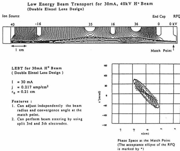
Fig. 5 Low energy beam transport for 30 mA, 40 kV H<sup>+</sup> beam.
