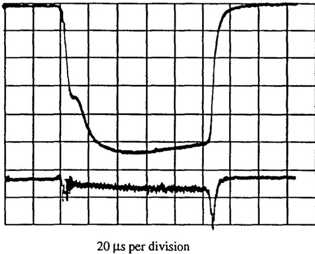
Fig. 3 Oscilloscope traces showing an  $H^-$  current of 100 mA. Top trace:  $H^-$  current, 20 mA per division, bottom trace: electron current, 500 mA per division.
