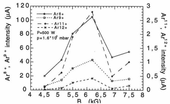
Fig. 3 - The current of high charge states for Argon vs.  $B_2$ .
