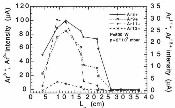
Fig. 6 - The current of high charge states for Argon vs.  $L_p$ .
