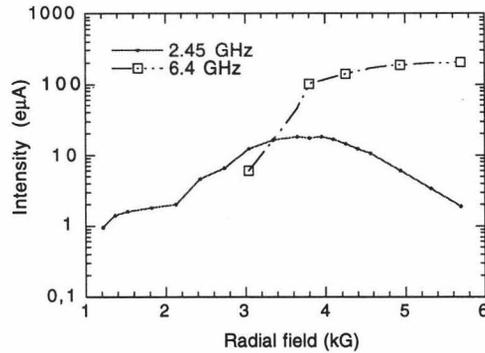
Fig. 7 - O<sup>6+</sup> current vs. B<sub>rad</sub> at 2.45 GHz and 6.4 GHz.
