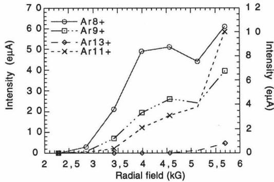
Fig. 4 - The current of high charge states for Argon vs.  $B_{rad}$ .
