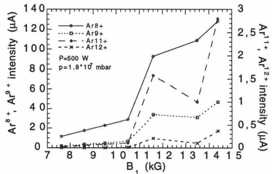
Fig. 2 - The current of high charge states for Argon vs.  $B_1$ .
