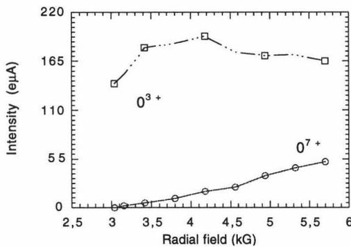
Fig. 5 - Measured current of  $O^{3+}$  and  $O^{7+}$  vs.  $B_{rad}$ .
