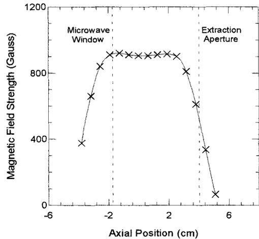
Figure 3: Axial Magnetic Field Profile of Permanent-Magnet Heavy Ion Source
