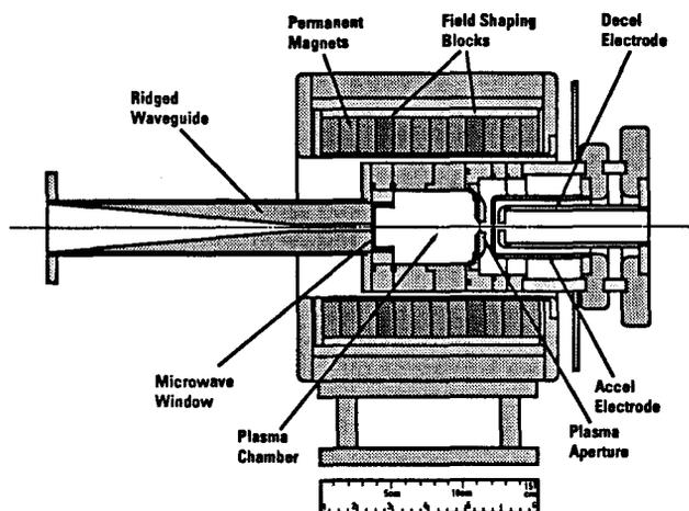
Figure 4: Compact Permanent-Magnet Microwave-Driven Ion Source
