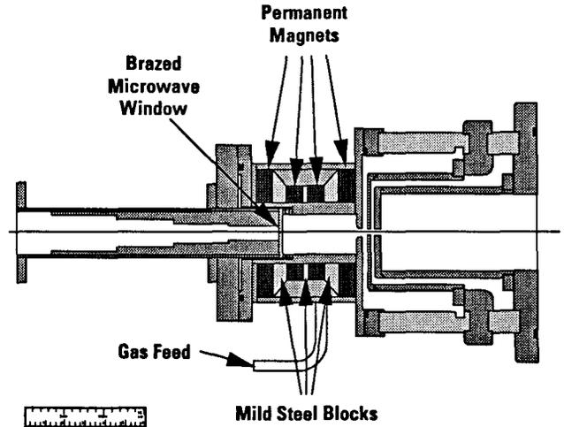
Figure 2: Permanent-Magnet Microwave-Driven Heavy Ion Source
