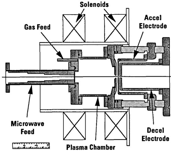
Figure 1: Microwave-Driven Chalk River Proton Source
