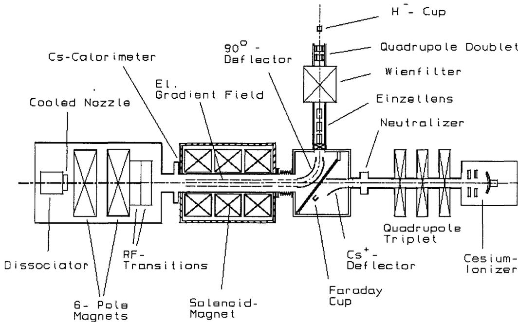
Figure 1: The polarized ion-source for COSY.
