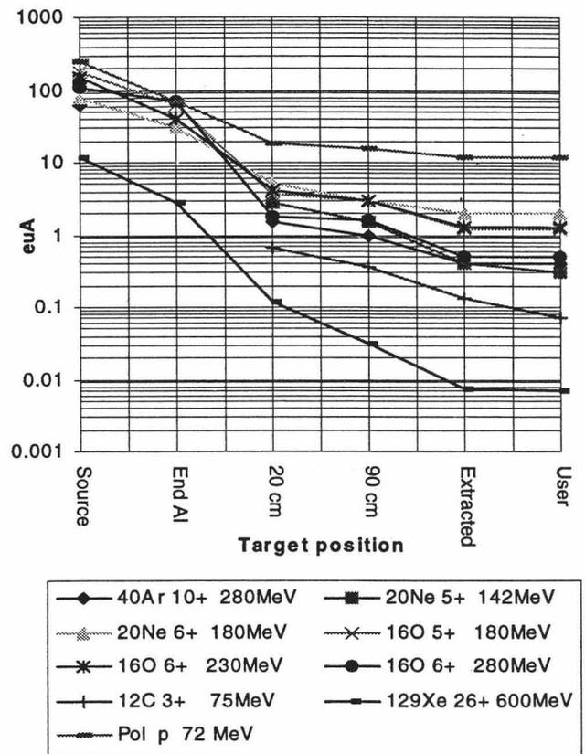
Fig. 4: Beam intensities at different targets and beam radii along acceleration path. When contamination from the Helium or Oxygen buffer gas is present interpolated values are given at the source and extrapolated ones at 20 cm. For Xenon the results are extrapolated to an isotopically pure target. The transmission observed with a proton beam from the polarized ion source is also shown for comparison.
