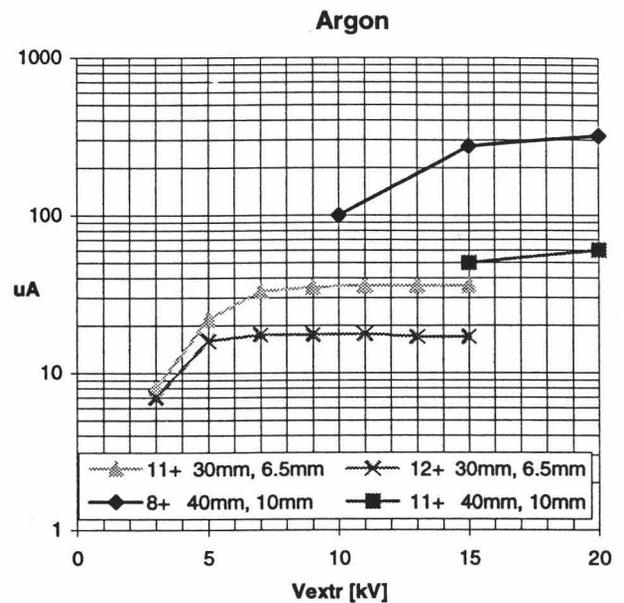
Fig. 2: Beam intensity as a function of the extraction voltage for different charge states and two extractor geometries. The distance between plasma and extraction electrodes and the plasma electrode aperture are indicated. For the measurements with the charge states 11+ and 12+ the source was optimized on state 11+ at 7 kV. The results at 20 kV are from the tests at Grenoble.
