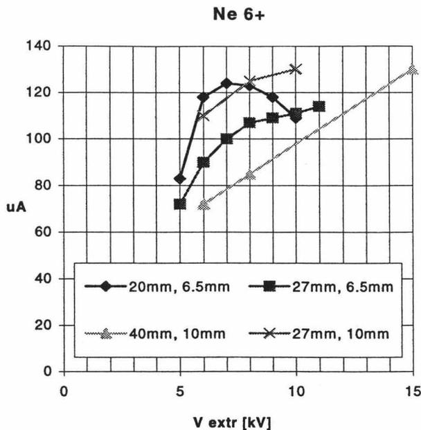
Fig. 3: Influence of the source extraction system on the beam intensity. The intensity of a Neon beam of charge 6+ is plotted for different separations of the electrodes and two diameters of the aperture of the plasma electrode. For the measurements with the 10 mm aperture the source was optimized at each extraction voltage, in the other cases it was optimized at 7 kV.
