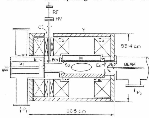
Fig 3. Schematic of modified ECR. Y-iron yoke, C1-C3 - Mag. coils, S1 - Stage one, S2 - Stage two, M - Sextupole, WN - Window, W - Water line, P1 - P2 - Pumps, Ex - Extractor, B - aluminum baffle plate, EE - Aluminum emission electrode
