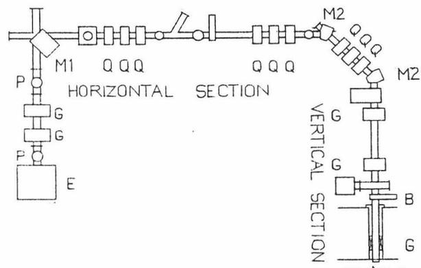
Fig 5. Schematic diagram of Injection line E - ECR ion source, P - Pump, G - Glaser, M1 - Analysing magnet, M2 -  $45^\circ$  bending magnet, B - Buncher, I - Inflector
