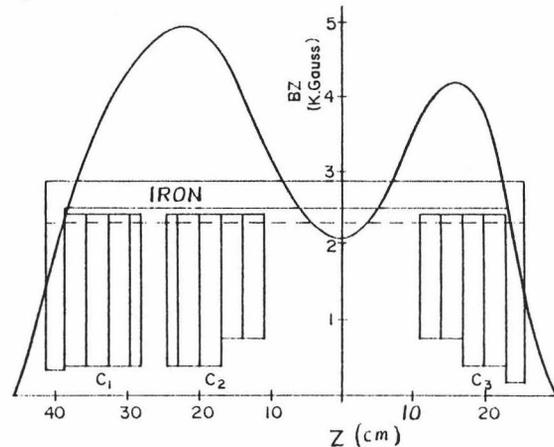
Fig - 4. Axial magnetic field distribution after adding extra coil.
