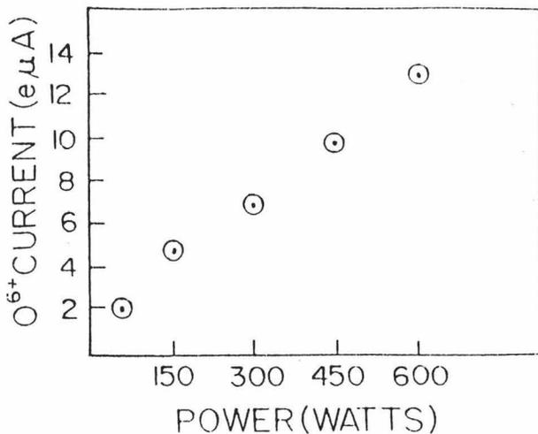
Fig 8. Ion beam current variation with RF power
