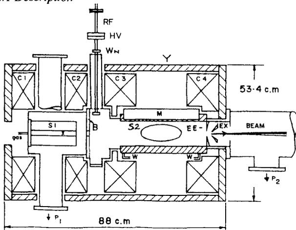
Fig 1. Schematic diagram of VEC ECR ion source. Y - Iron Yoke, C1 - C4 - Mag. coils, S1 - Stage -1, S2 - Stage 2, M - Sextupole, WN - Window, W - Water line, P1 - P2 Pumps, EX - Extractor, B - Baffle plate, EE - Emission electrode.
