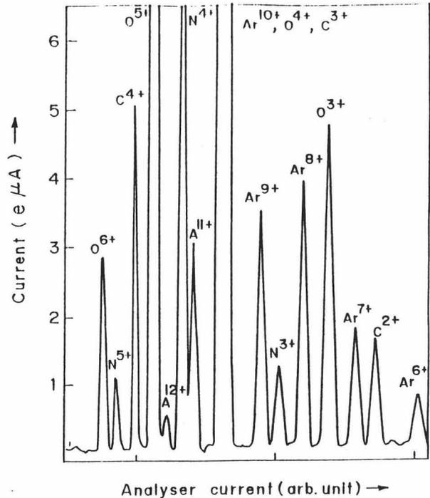
Fig. 7. Spectrum of Argon charge states, Tuned for Ar<sup>11+</sup>
