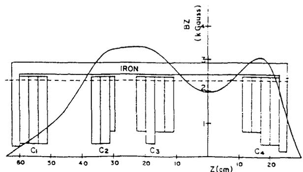
Fig 2. Axial Magnetic field of the solenoidal coils with gradient configuration in the first stage for 6.4 GHz operation. Excitation current in coil C1 is zero in this case
