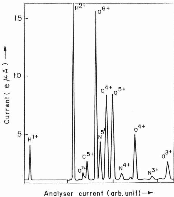
Fig. 6. Spectrum of Oxygen charge states, tuned for O<sup>6+</sup>
