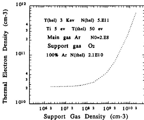
Figure 2: Dependence of the thermal electron density on the support gas density
