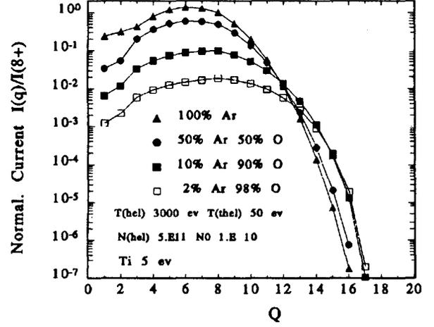
Figure 1: Charge state distribution for different mixing ratios between the main gas and the support gas. All the ion currents are normalized to the currents of  $A_r^{8+}$  without support gas.
