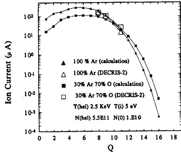
Figure 3: Comparison between the calculated charge state distributions and the experimental measurements from DECRIS-14-2 for argon mixed with oxygen.
