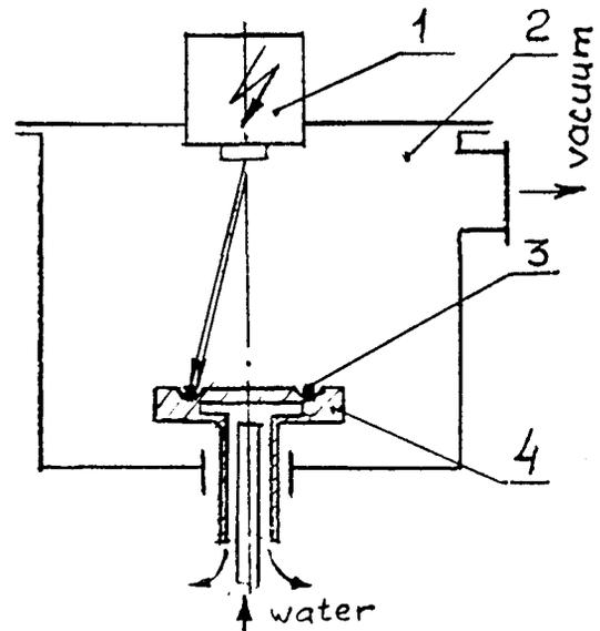
Fig.1. The scheme of the electronic beam gun set up.
