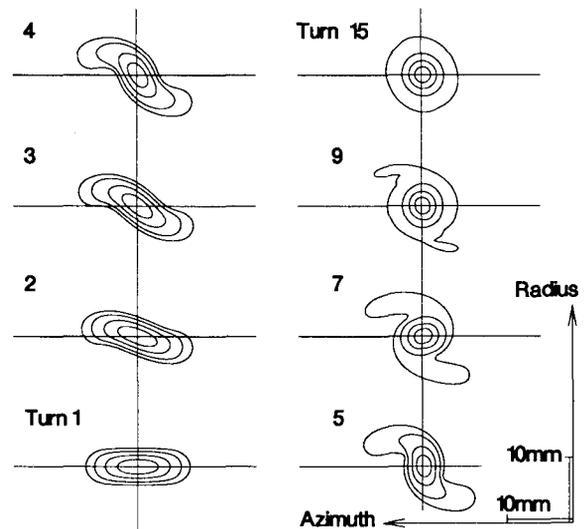
Figure 1: Simulation of the evolution on the first few turns in the PSI injector 2 cyclotron of a 1.0 mA beam bunch starting with a phase width of 15 degrees. Within 5 to 10 turns a round charge distribution is formed due to space charge forces. The contour lines represent 10%, 20%, 50% and 80% of the maximum charge density.
