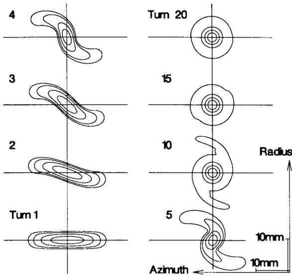
Figure 2: Simulation of a coasting beam of 1 mA with the Sphere Model. A beam bunch of initially 15 degrees phase width, remaining on 3 MeV without acceleration is deformed into a galaxy shaped charge distribution within 5 to 10 turns.
