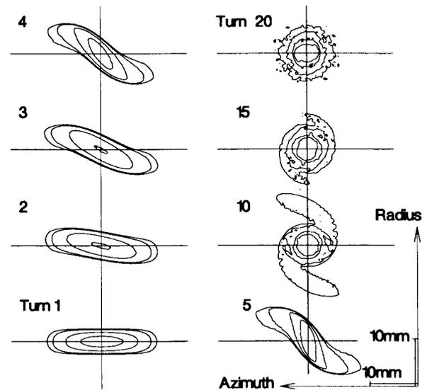
Figure 3: Simulation of a coasting beam of 1 mA with the Needle Model, remaining at 3 MeV in the injector 2 cyclotron. From the initial phase width of 15 degrees the beam bunch is deformed into a galaxy shaped charge distribution within 5 to 10 turns.
