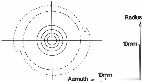
Figure 4: The formation of a "round" charge density distribution due to space charge forces is accompanied by the production of wide haloes. For turn # 40 of a 3 MeV coasting beam with 1 mA and initially 15 degrees phase width the 1% (dotted) and 2% (dashed) contours are shown in addition to the full lines for 10%, 20%, 50% and 80% of the maximum charge density.
