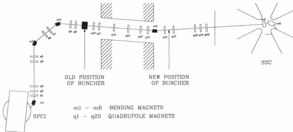
Fig 1 Layout of the injection beamline between SPC1 and the SSC with the old and new buncher positions indicated.
