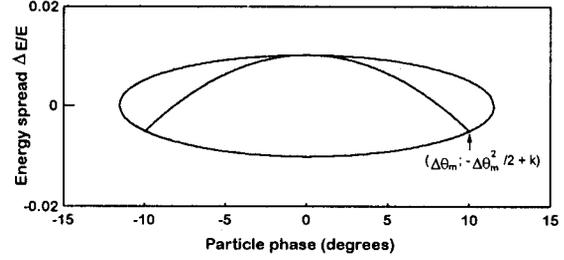
Fig 2 An ellipse which includes all the particles in a beam pulse with pulse length of  $20^\circ$ . The half-axes of the ellipse are  $\Delta\theta = \frac{2}{\sqrt{3}} \Delta\theta_m$  and  $\Delta E/E = \Delta\theta_m^2/3$ .
