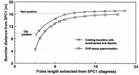
Fig 4 The optimum buncher position, for minimum radial beam width at extraction in the the SSC, as a function of the beam pulse length at the start of the injection beamline.
