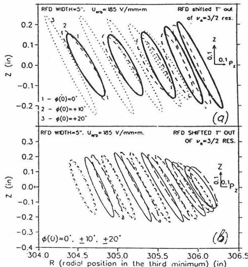
Figure 6: Vertical ellipses for turns in the extraction region (third precession minimum).  $\delta\phi = 40^\circ$ . The phase dependence in the orientation of the stretched ellipses evident in (a) is absent in (b) by the addition of a flattopping voltage.(Improved RFD design)
