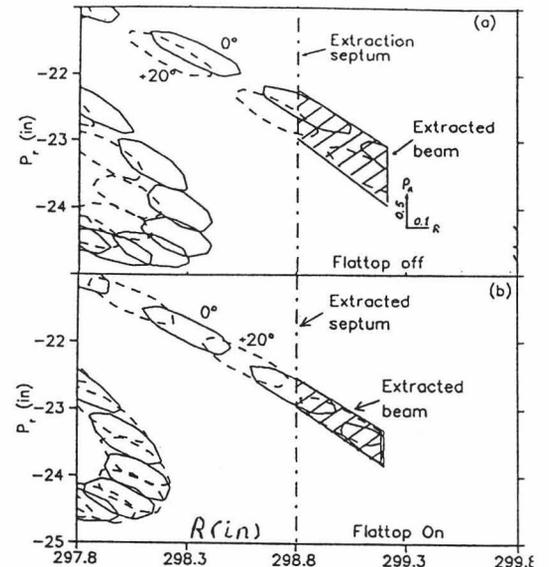
Figure 8: Position in radial phase space of a matched beam ellipse undergoing precession extraction for two different starting phases,  $0^\circ$  and  $+20^\circ$ . (a) NO FLATTOP. In (b) a 4<sup>th</sup> harmonic FLATTOPPING voltage has been added to the accelerating field reducing the variation in precession between different RF phases. The hatched region represent the area in radial phase space occupied by the extracted,  $40^\circ$  wide, beam.
