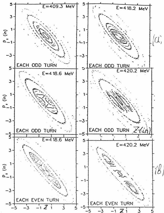
Figure 5: Vertical Phase Space diagrams. Original RFD device is ON: (a)- each odd turn, (b) - each even turn.
