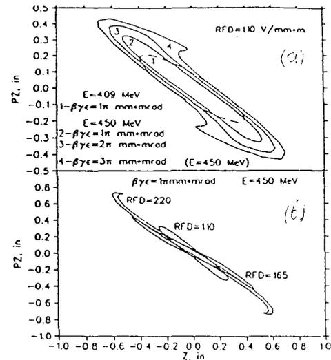
Figure 4: Comparison of vertical ellipse shapes: (a) for different values of initial emittance; (b) for different RFD strength.
