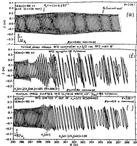
Figure 3: Vertical phase ellipses. Center of each ellipse corresponds to the radius of given turn: (a) RFD is OFF; (b) Original RFD design. Ratio of stretched vertical amplitude to initial one is  $A_z(str)/A_z(init) = 1.85$ ; (c) Improved RFD design.  $A_z(str)/A_z(init) = 1.28$ . Ratio of stretching is reduced on 50%.
