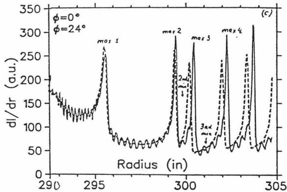
Figure 1: Radial scans using a differential probe showing the beam density pattern produced by the RFD for an optimized phase band and for a phase band off-set by 24°. Phase dependent amplitude growth at the  $\nu_r=3/2$  account for the difference.
