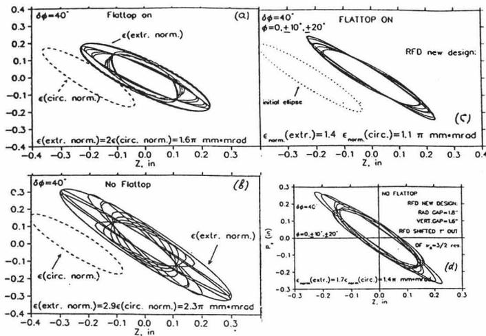
Figure 7: Extracted vertical emittance as a superposition of vertical phase ellipses for different initial RF phases ( $\Delta\phi = 40^\circ$ ). Original RFD design: (a)FLATTOP ON; (b)FLATTOP OFF. Improved RFD design: (c)FLATTOP ON; (d)FLATTOP OFF
