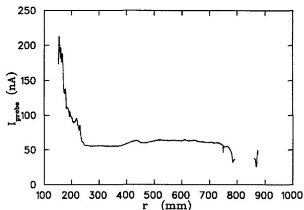
Figure 3: Accelerated beam current measured on the main probe
