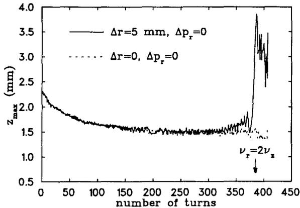
Figure 4: Effect of radial off-centering on the beam vertical size at the Walkinshaw resonance location
