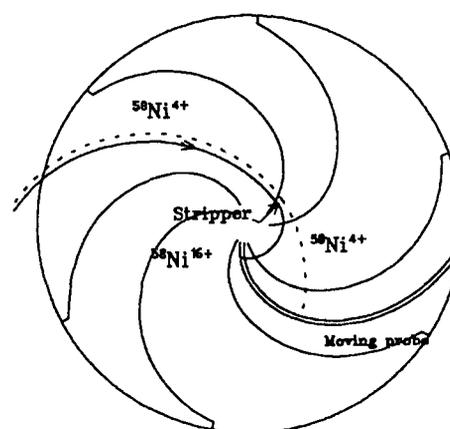
Figure 1: Pole region of the Catania Superconducting Cyclotron
