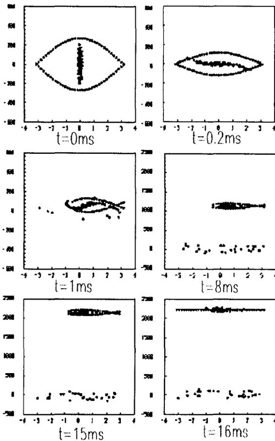
Figure 2: The simulation of momentum phase space evolution. (horizontal: RF phase, vertical:  $\delta PC$ )
