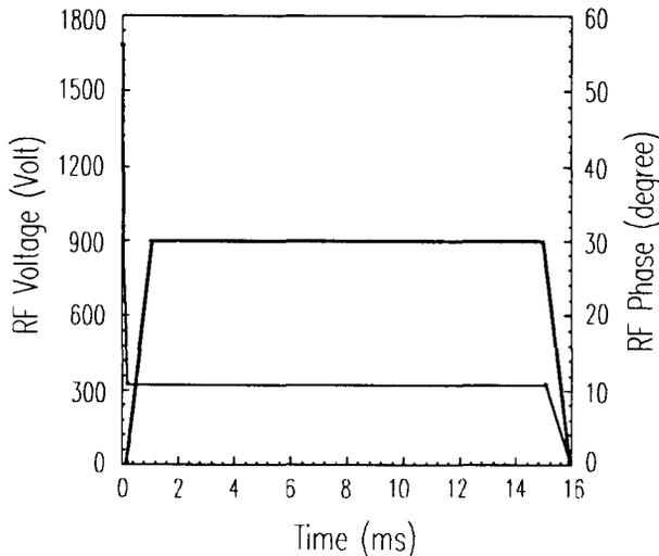
Figure 1: The parameters of RF system. (thin line: RF voltage, thick line: RF phase)
