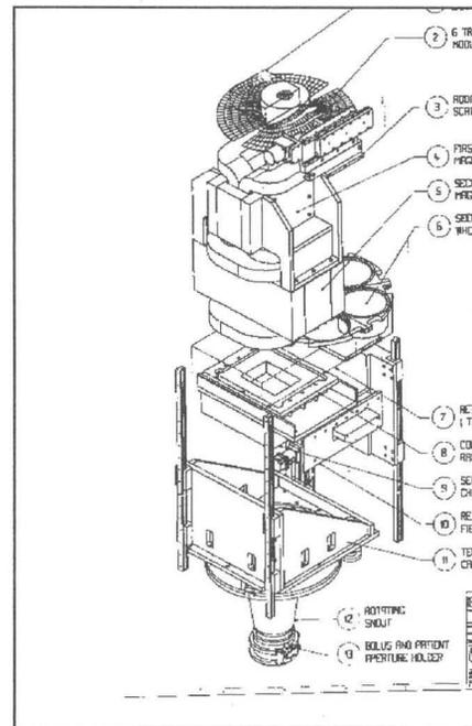
Figure 3. Schematic of Nozzle Components
