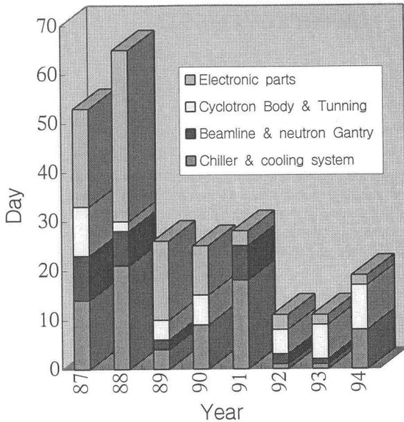
Figure 4: Failure days and parts
