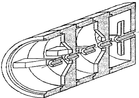
Figure 2: H-resonator with drift tubes and crossed holders. Drift tubes are fasten on holders, revolved for next drift tubes on a corner, close to 90 grades. In first and last half-cells of H-resonator, cross-shaped tuning elements may be placed. Another name this accelerator is IH type linac,
