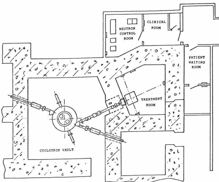
Fig.1 GENERAL LAYOUT OF NEUTRON THERAPY FACILITY
