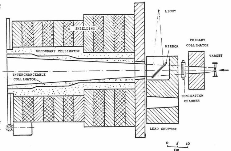
Fig.2 COLLIMATOR SYSTEM AND TARGET
