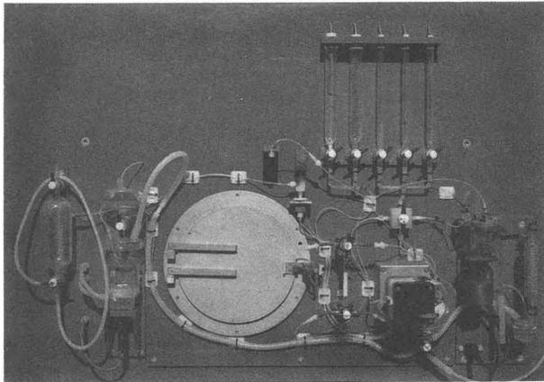
Figure 1: System for recovery of <sup>67</sup>Ga from Zn targets.
