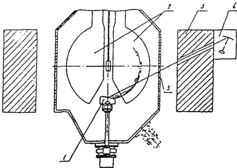
Figure 1 : Plane view of internal target position in IPPE cyclotron : 1 - target, 2 - dees, 3 - magnet yoke, 4 - infrared radiometer, 5 - window passing infrared radiation
