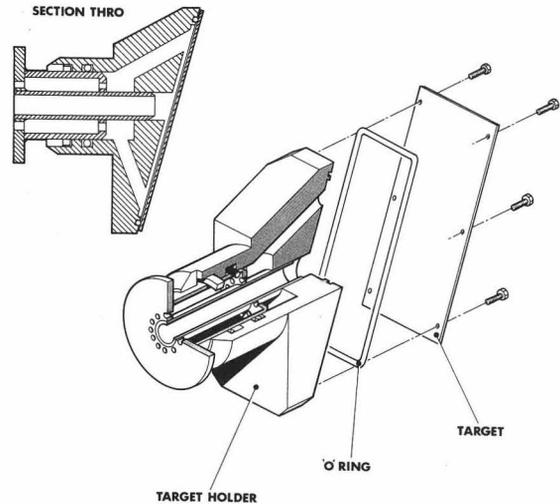
Figure 3: A three dimensional view of the modified target assembly. The scale is noted. The water cooling enters into the center of the target plate and exists at either end of the target head assemble through 0.25 inch ports.
