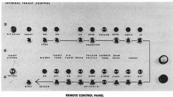
Figure 2: The Remote Control Panel, located in the main control room, showing push buttons for manual operations and the sequence of operations as indicated by the direction of arrow.
