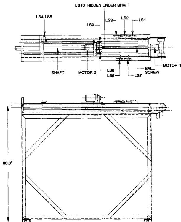
Figure 1: A schematic view of the aluminum stand, angle aluminum, stainless steel shaft, drive mechanism and various microswitch to control different stages of target from loading to the stage of irradiation and back after irradiation. M = Servo motor, LS = limit switches.
