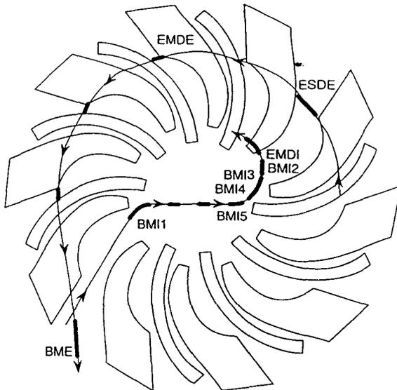
Fig. 6: Injection and extraction channels of the BSSC
