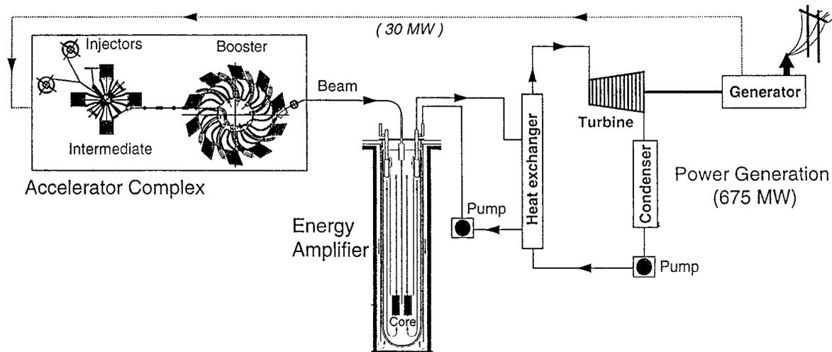
Fig. 1: Schematics of the Energy Amplifier complex
