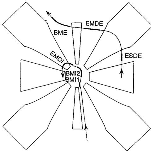
Fig. 4: Injection and extraction system of the ISSC
