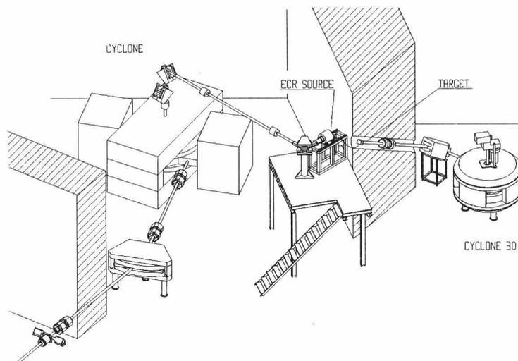
Figure 1 : Layout of the present radioactive beam facility
