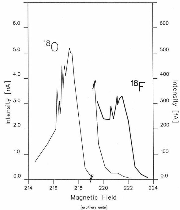
Figure 2 : Isobaric separation of  $^{18}\text{O}$  and  $^{18}\text{F}$  : intensity of the extracted beam versus the magnetic field of the cyclotron. Note that the intensity scale is different for  $^{18}\text{O}$  (left scale, nA) and for  $^{18}\text{F}$  (right scale, fA)
