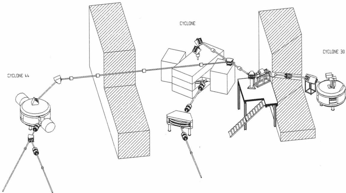
Figure 3 : Layout of the future radioactive beam facility
