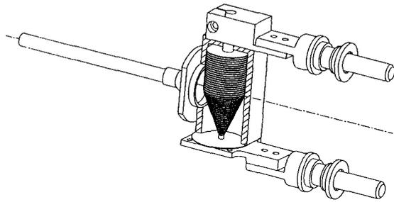
Fig. 4 : Structure of the conical target
