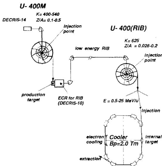
Figure 4: The conceptual view of U400M–U400 facility.
