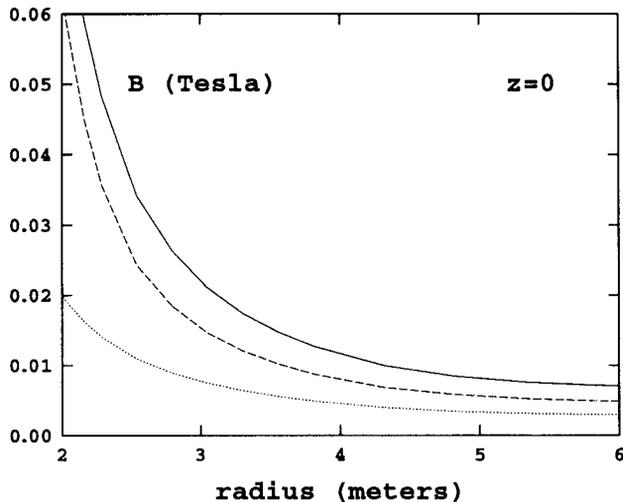
Figure 2: Poisson computations of median plane fringe fields for 1) the MSU K500 cyclotron as it now exists (the solid curve), 2) the K500 with an additional 10 cm layer of steel added on top, bottom, and outer periphery of the magnet (the dashed curve), and 3) with the further step of filling the coil support holes in the median plane and on the top and bottom of the cyclotron with iron (the dotted curve).
