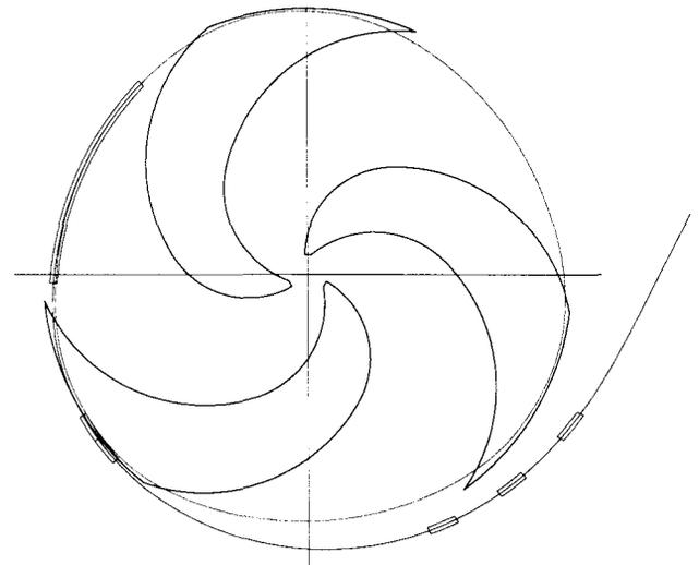
Figure 5: Extraction orbit of the modified MSU K500 at the 200 MeV proton operating point. The electrostatic deflector inside the dee at the upper right operates at 125 kv/cm and five magnetic channels of 6 degree length with a gradient of 32.7 T/m and 0.13 T dipole field i.e. the same values as present K500 magnetic channels.
