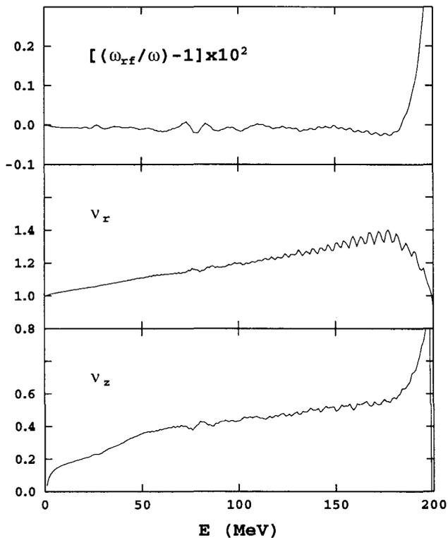
Figure 4: Orbital frequency and transverse oscillation frequencies for the 200 MeV proton operating point of an MSU K500 in which the magnet gap is reduced to 16mm near the magnet edge and the yoke has an additional 10 cm layer of steel (as in the dashed curve of Figure 2).
