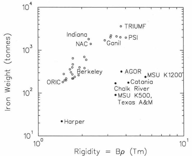
Figure 1: Iron weight in metric tonnes vs. maximum bending power in tesla meters for the large cyclotrons in the world. Numerical values are from the “Data Sheets” given in Proceedings of the Thirteenth International Conference on Cyclotrons and Their Applications, Vancouver 1992.
