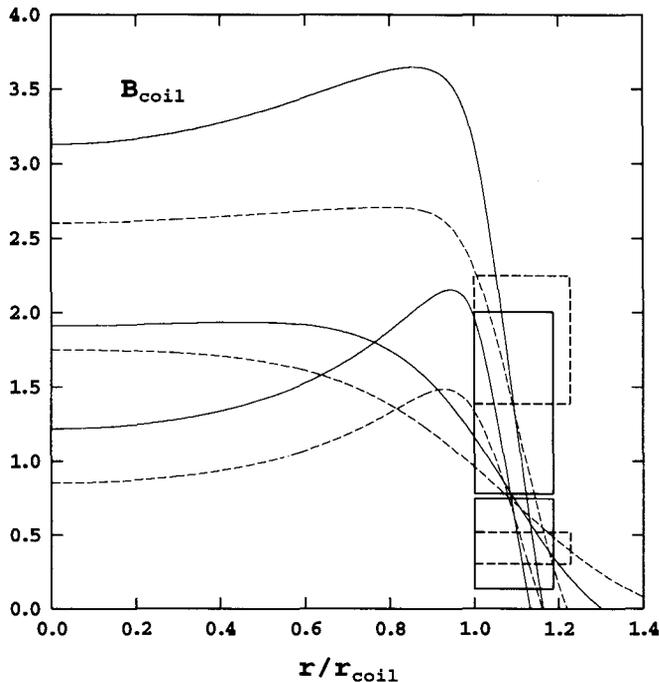
Figure 3: Air-core calculations of the magnetic field of the main coils of the Agor cyclotron (dashed lines) and of the MSU K500 (solid lines). The three curves are in each case for the individual coil and for their sum, with current in all cases at peak design values. Dashed and solid boxes show the physical shape of the coils.
