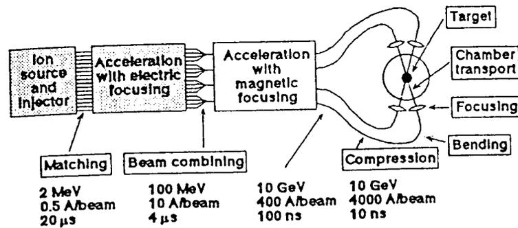
Figure 3: The multiple-beam heavy ion induction linac concept. The shaded areas indicate driver areas that have been investigated by technology developments and/or model physics experiments.
