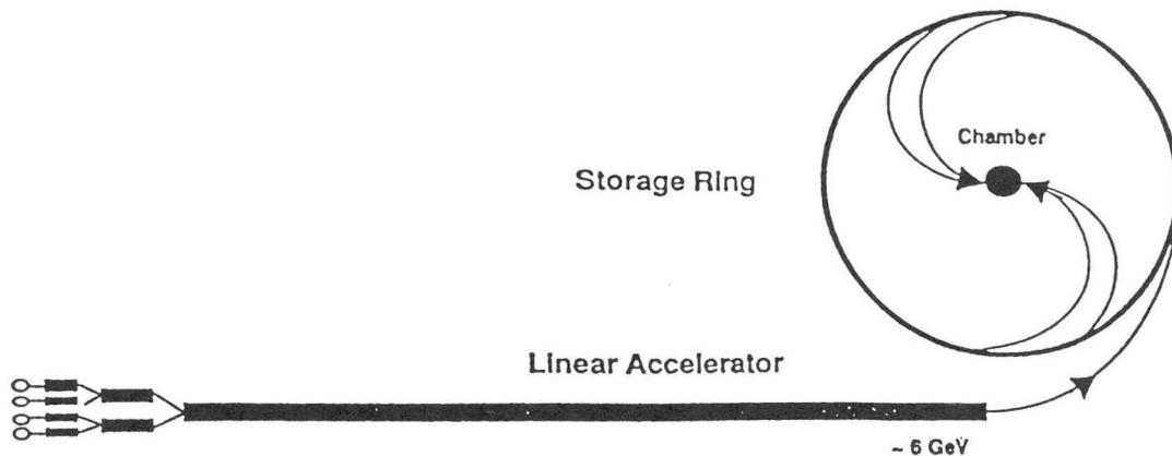
Figure 8: Concept of a heavy ion driver accelerator for an ignition test facility (I. Hofmann *et al.* [4])
