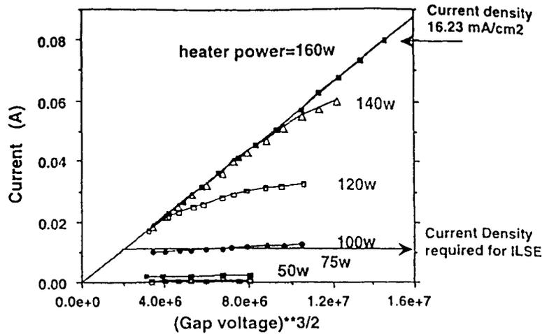
Figure 4: Measurements of Potassium<sup>+1</sup> emission from a zeolite ion source as a function of applied voltage and heater power [5]
