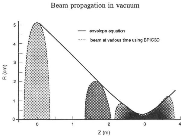
Figure 7: Comparison of the envelope equation and the BPIC3D code results for the propagation of the beam through a vacuum. The beam is plotted at six successive times.
