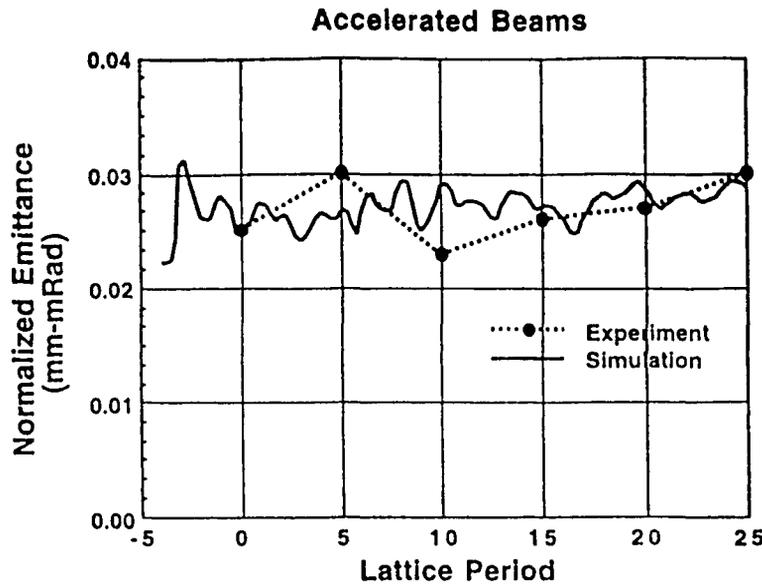
Figure 6: Measurement and simulation of the normalized emittance of a  $\text{Cs}^{+1}$  beam during acceleration through MBE-4. With care acceleration and current amplification were achieved with no degradation in beam quality.
