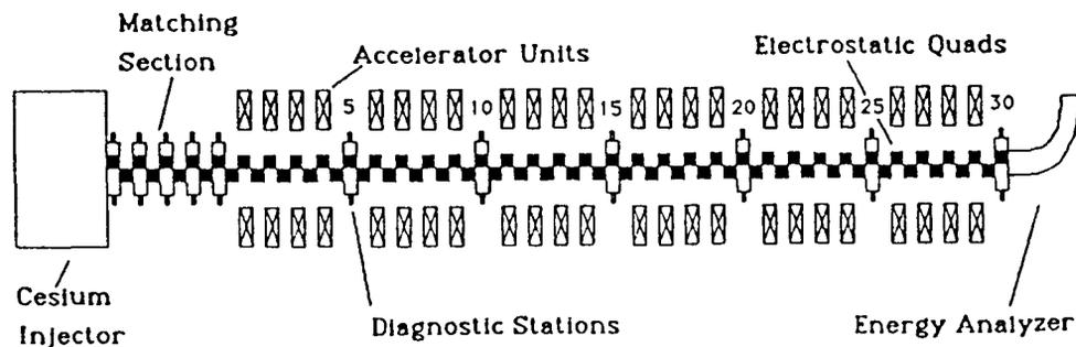
Figure 5: Schematic of the MBE-4 current amplifying induction accelerator
