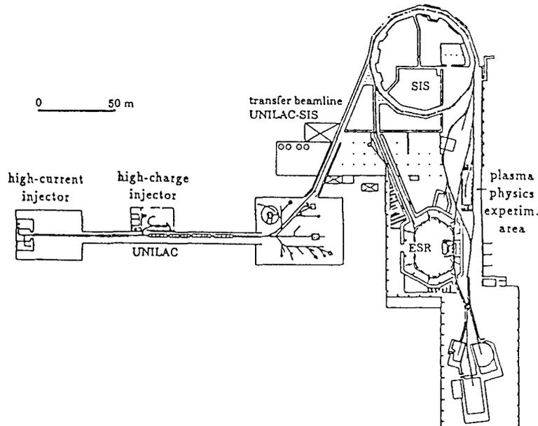
Figure 2: The GSI 2-ring heavy-ion accelerator facility SIS/ESR with UNILAC as an injector for all ion species up to Uranium. The injector energy is 11.9 MeV/u, the maximum energy of SIS 2 GeV nucleon. Ions can be stored and cooled (up to  $10^{10}$  ions) in the ESR and reinjected in the SIS. The target cave on the right hand side is dedicated to beam-target interaction experiments.
