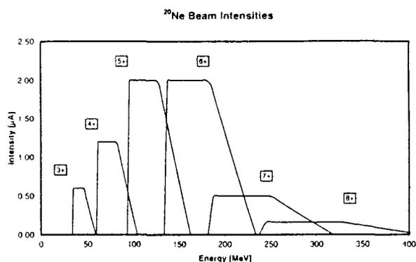
Figure 2: Predicted  $^{20}\text{Ne}$  beam intensities in the energy range of the PSI Philips Cyclotron.
