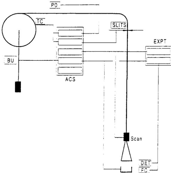
Figure 3: Feedback system for the control of the beam stability. Signals from the phase detector (PD) or from slits are used to apply field corrections with the outermost trimcoil (TC). The variation of the buncher voltage (BU) eliminates current instabilities. The signals from a Faraday cup (FC) or from monitor detectors (DET) are processed by the experiment and/or the Accelerator Control System. The last steering magnet can also be used for beam scanning.
