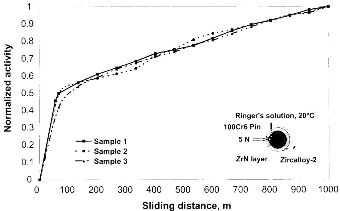
Fig. 4 : Normalised summed activity in collection buffer bottle versus sliding distance during wear testing of 3 different samples of nitrided Zircalloy-2.
