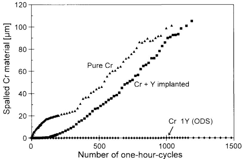
Fig. 1 Spallation behaviour measured using TLA of pure Cr, Cr implanted with  $10^{17}$  Y-ions/cm<sup>2</sup>, and Cr-1%Y<sub>2</sub>O<sub>3</sub> alloy upon thermal cycling at 1000°C [7].
