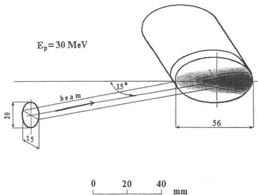
Fig.3. Layout of internal target irradiation
