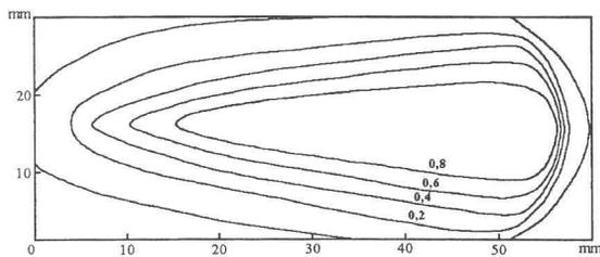
Fig.4. Current density distribution across isotope target surface.
