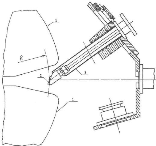
Fig. 2. Schematic view of the target position in the cyclotron tank.
