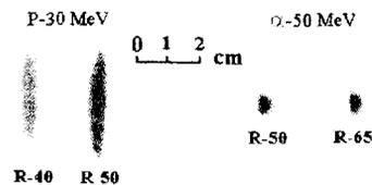
Fig.1 Beam spots for different particles and energies.
