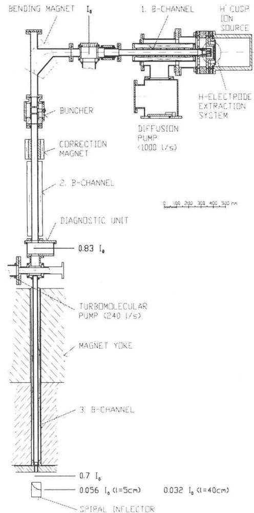
Figure 2. Layout of the axial injector with the transmission coefficients (buncher OFF)
