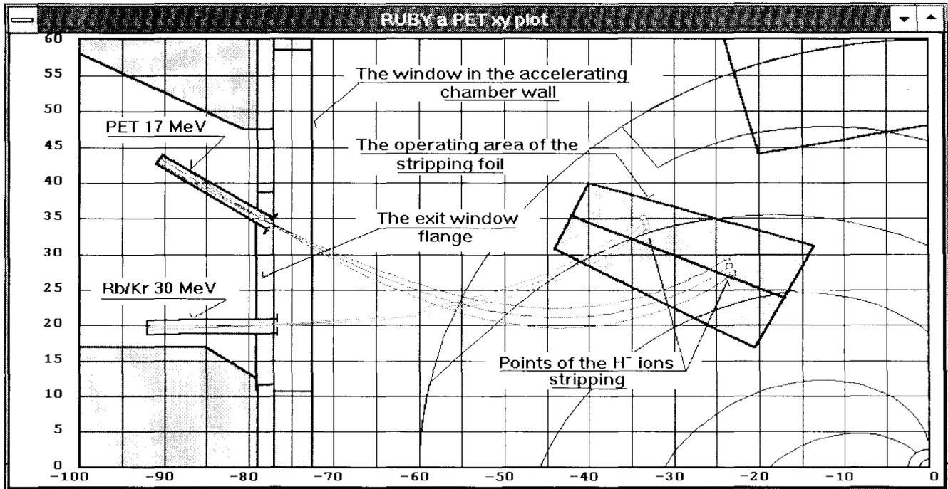
Figure 3. Extraction of the 17MeV and 30MeV protons
