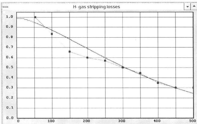
Figure 1. H<sup>-</sup> gas stripping beam losses with internal ion source
