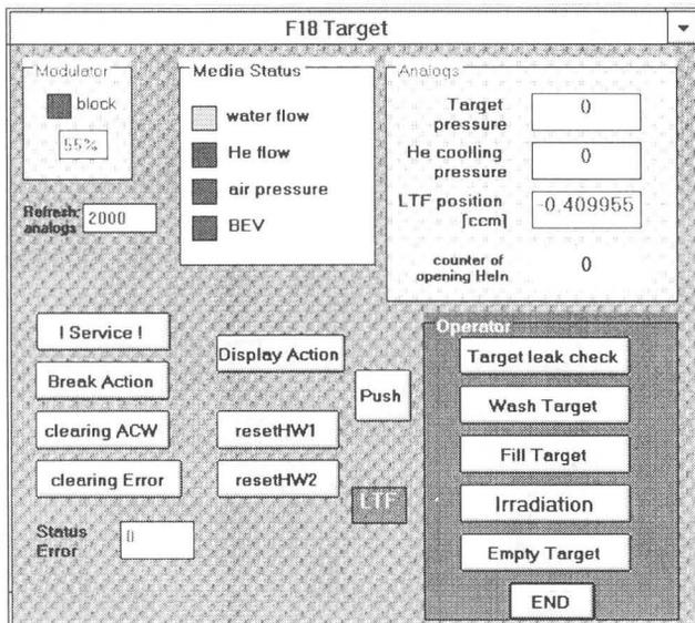
Figure 4.  $^{18}\text{F}$  target control panel
