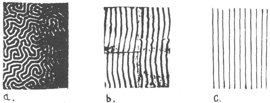
Fig. 2. Microphotograph of domain structures of BGF.
