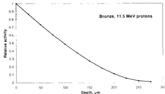
**Figure 2** Relative  $^{65}\text{Zn}$  activity versus depth for protons of 11.5 MeV in natural Cu-5wt%Sn measured experimentally using the stacked-foil technique.
