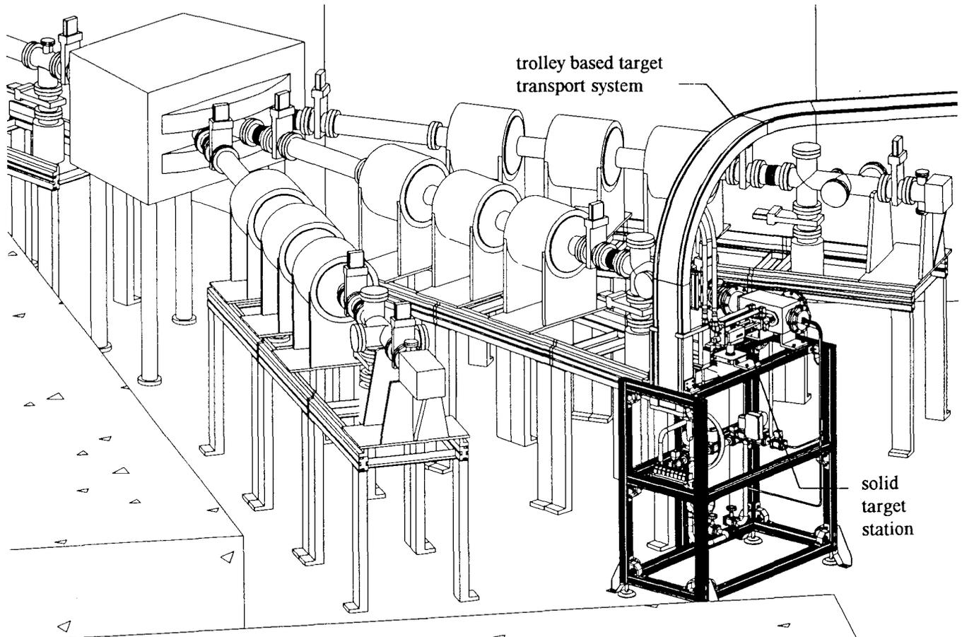
Figure 2: The solid target station positioned in the target area of the channel for production of radioisotopes.
