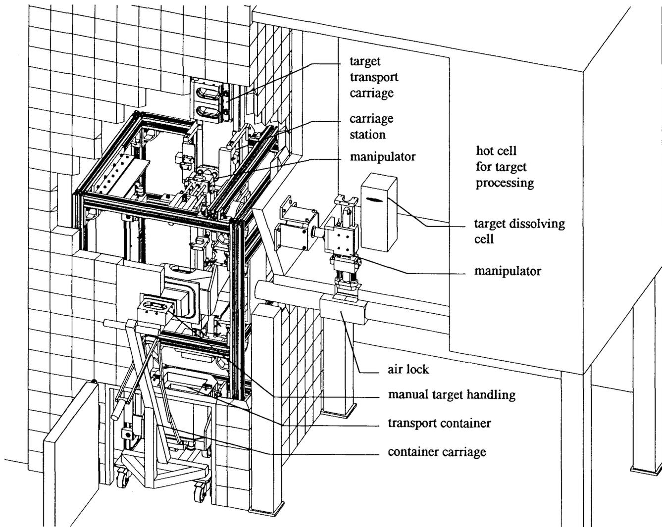
Figure 4: Service station for target handling
