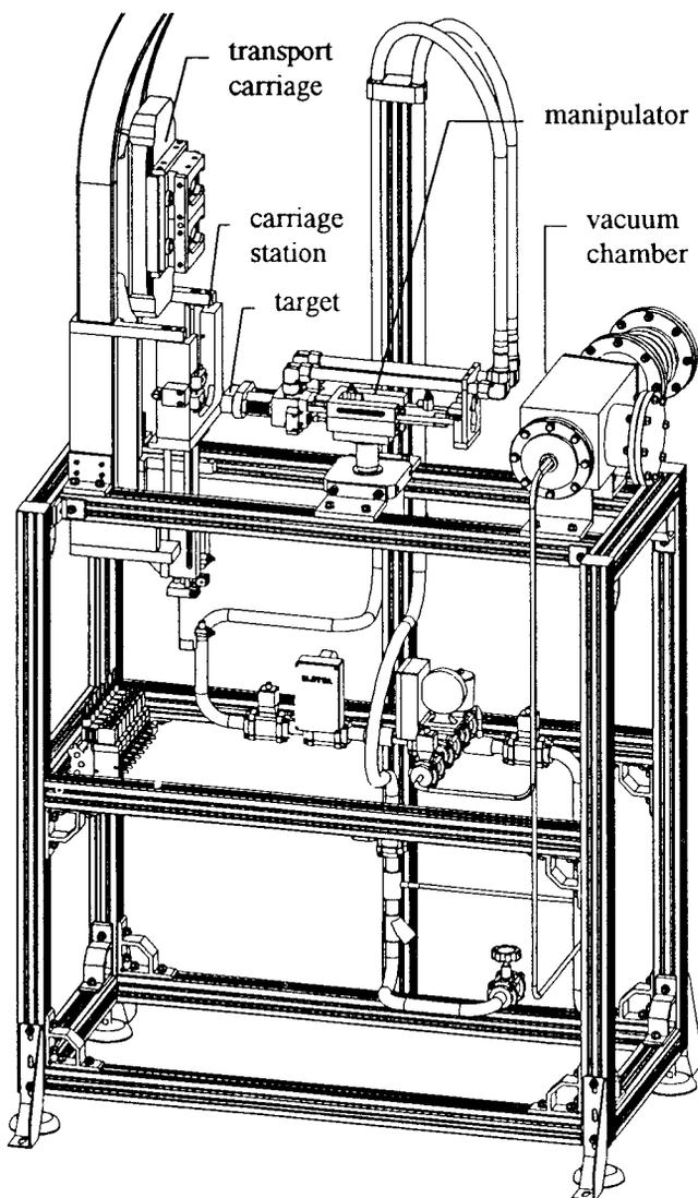
Figure 3: The solid target station
