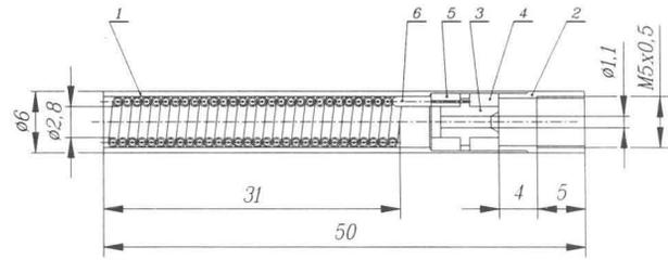
Figure 4: Microoven. 1,2 - body, 3 - electrical connector, 4,5 - ceramic insulators, 6 - heater.
