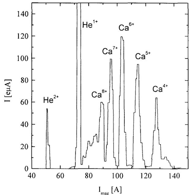
Figure 1: The  ${}^{48}\text{Ca}$  ion spectrum, optimised for  $\text{Ca}^{6+}$ .
