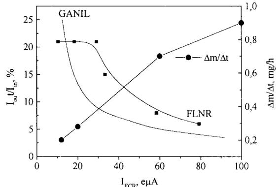
Fig.7 Experimental results for the bunching effect and consumption of metallic  ${}^{48}\text{Ca}$  versus the ion beam intensity from the ion source
