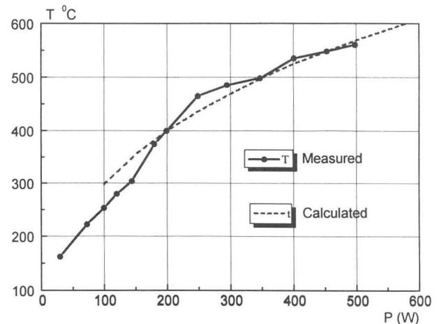
Figure 5: Measured and calculated screen temperature vs microwave power.
