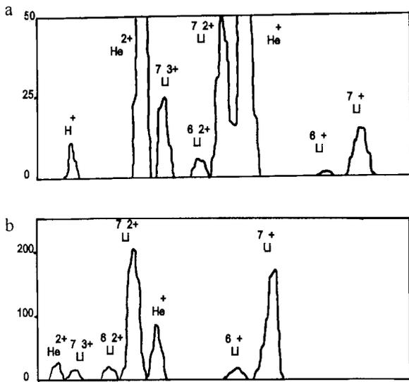
Figure 6: The Li ion beam spectrum, optimized for  $\text{Li}^{2+}$  (a - without a screen, b - with a screen).
