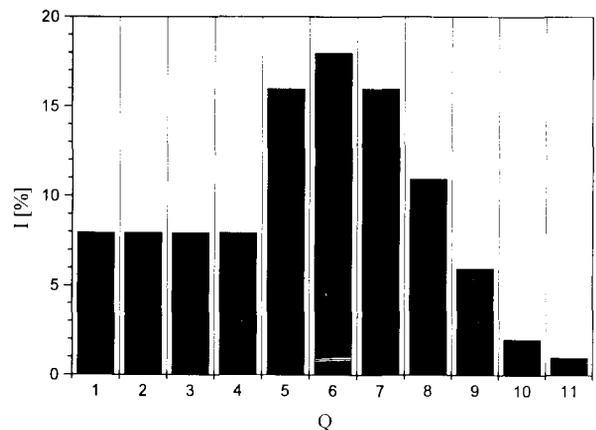
Figure 2: Number of particles, in percents, in the Ca ion beam for different charge states.
