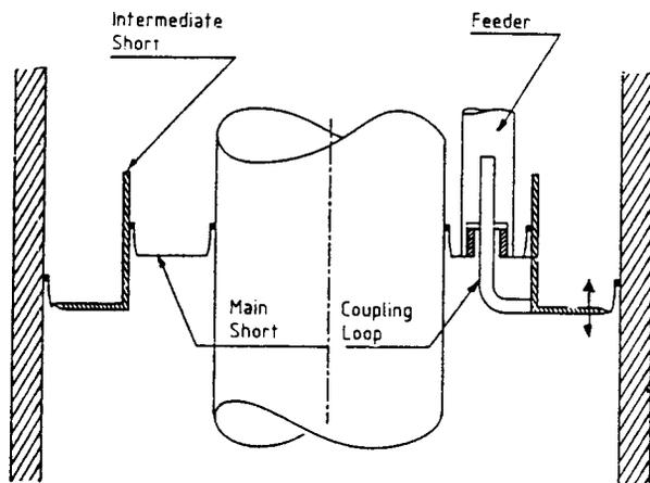
fig. 1 Schematic drawing of the sliding short and coupling loop
