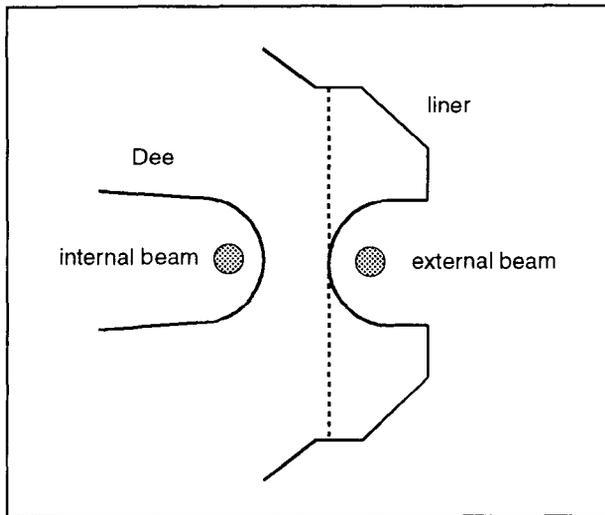
fig. 3 Geometry of Dee and liner of resonator 3; dashed line indicates modification to remove multi-pactor
