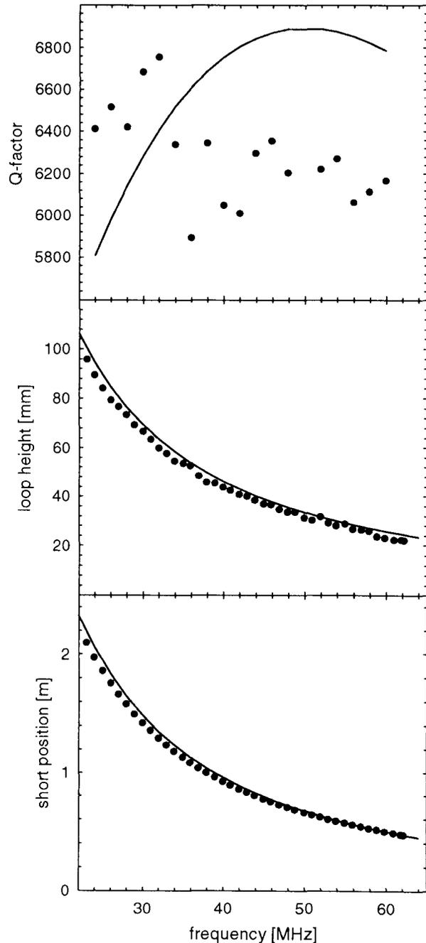
fig. 2 Resonator characteristics as a function of frequency
