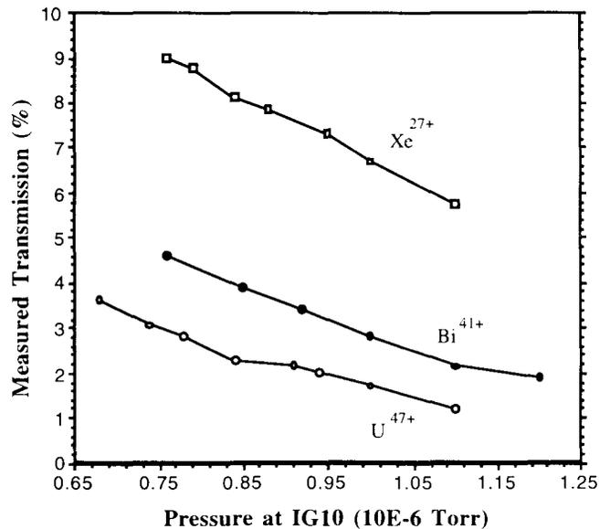
Fig. 4. Measured acceleration transmission versus pressure in the 88-Inch Cyclotron for  $\text{Xe}^{27+}$ ,  $\text{Bi}^{41+}$  and  $\text{U}^{47+}$  ion beams.
