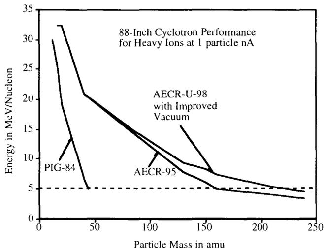
Fig. 1. This shows the energy-mass curves for the cyclotron at an intensity of 1 particle nA.
