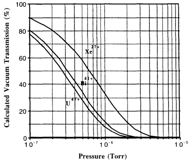
Fig. 6. Calculated beam vacuum transmission versus pressure for  $Xe^{27+}$ ,  $Bi^{41+}$  and  $U^{47+}$  ion beams accelerated by the 88-Inch Cyclotron. Improvement ratios are in good agreement with the measured data.
