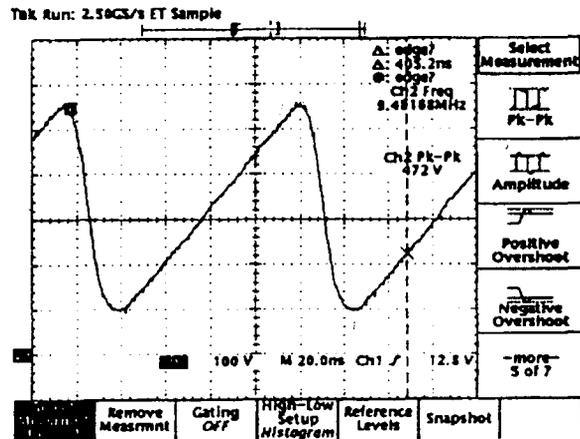
fig. 3 Sawtooth voltage generated with prototype electronics on a 20 pF capacitance
