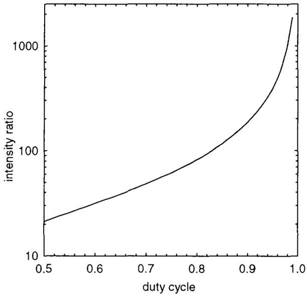
fig. 1 Intensity ratio between main and parasite pulses as a function of buncher duty cycle
