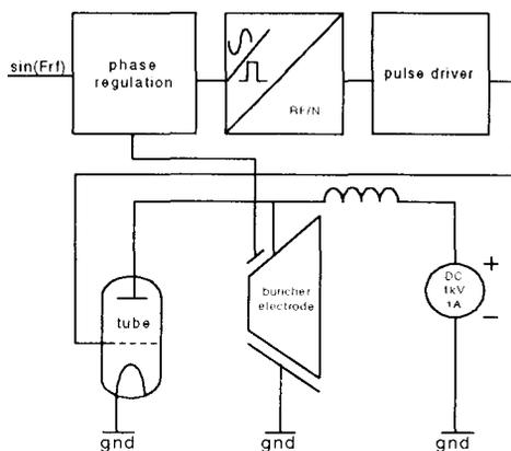
fig. 3 Block diagram of subharmonic sawtooth buncher
