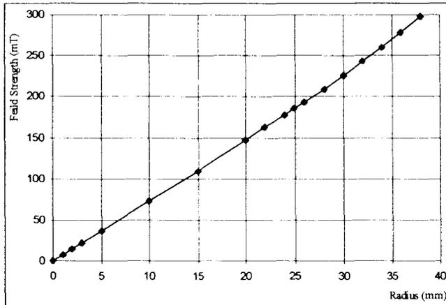
Figure 5: B vs radius inside magnet structure
