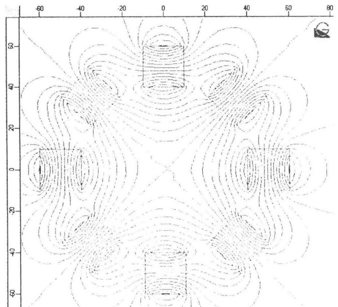
Figure 1: 2-D simulation showing flux lines of one of the tested configurations
