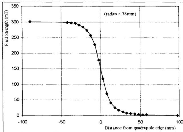
Figure 6: B vs z at 38mm radius
