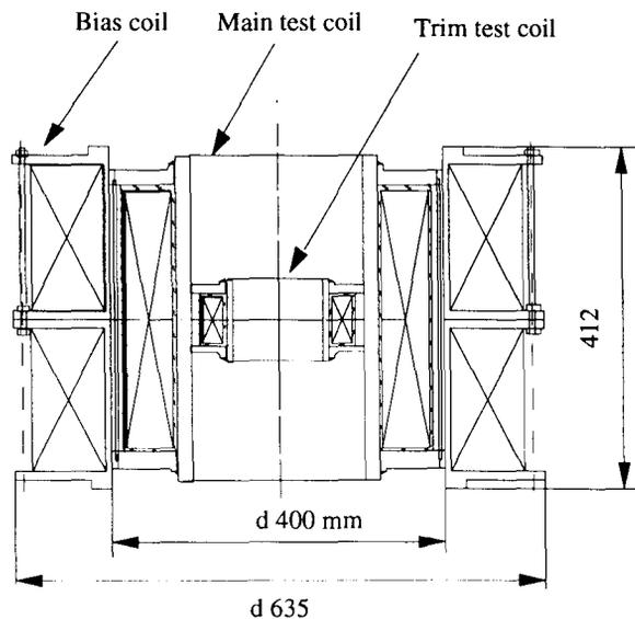
Fig. 4. Coils arrangement for the stabilizing test.
