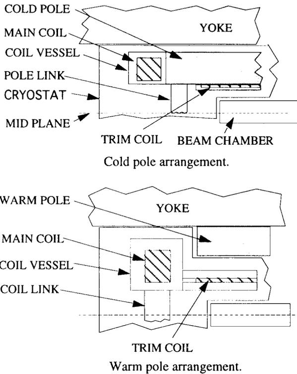
Fig. 2. Comparison of the pole arrangement.
