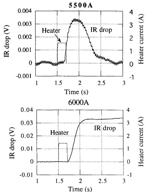
Fig. 5. Measured voltage drop change of the test main coil.
