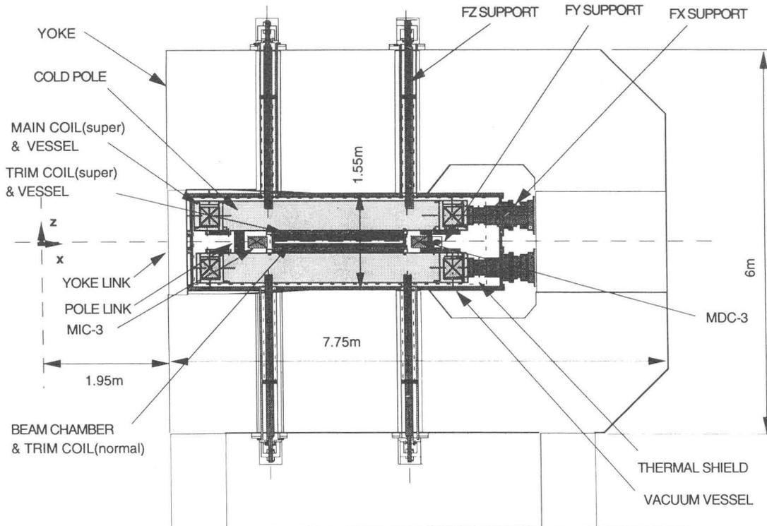
Fig.1. Cross-sectional view of the SRC sector magnet.
