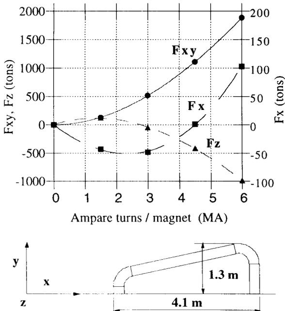
Fig. 3. Magnetic forces exerted on the cold mass.
