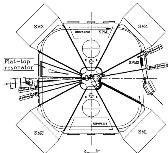
Figure 2: Layout of the SSC showing a flat-topping dee in the injection valley vacuum chamber.
