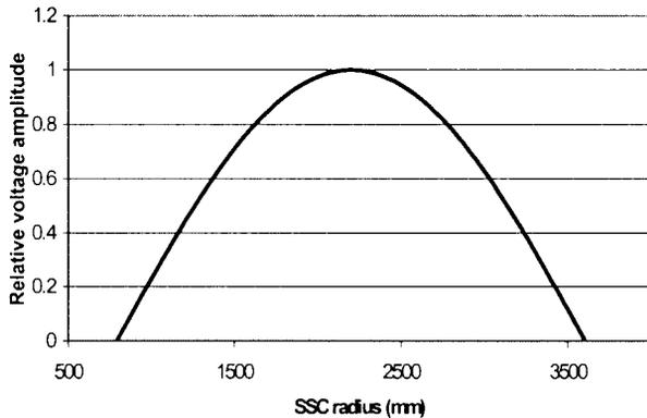
Figure 8: Dee voltage as a function of radius for the horizontal half-wave resonator.
