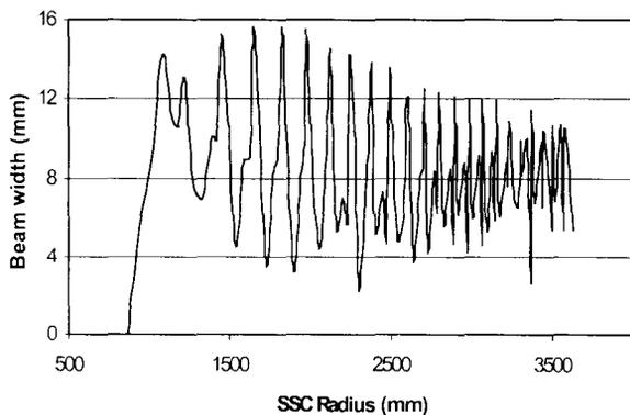
Figure 6: Beam width due to energy spread as a function of radius for a 40° long beam pulse and a vertical half-wave resonator.
