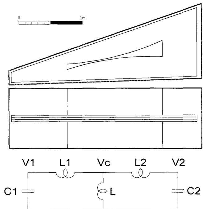
Figure 4: Top and side views of the resonator and the circuit diagram used to explain its characteristics.
