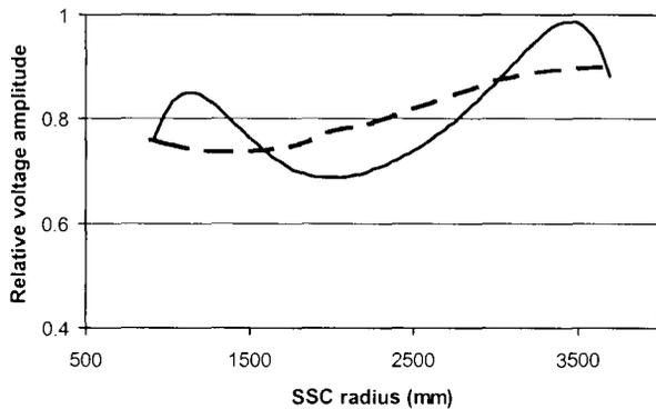
Figure 5: Dee voltage as a function of radius for the vertical half-wave resonator (solid line) and the SSC main resonators
