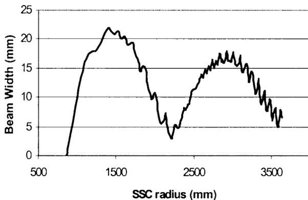
Figure 9: Beam width due to energy spread as a function of radius for a 40° long beam pulse and the horizontal half-wave resonator.
