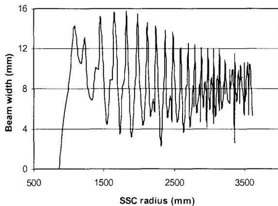
Figure 3: Beam width due to energy spread as a function of radius for a 40° long beam pulse with one flat-topping resonator and a voltage distribution identical to those of the main resonators.
