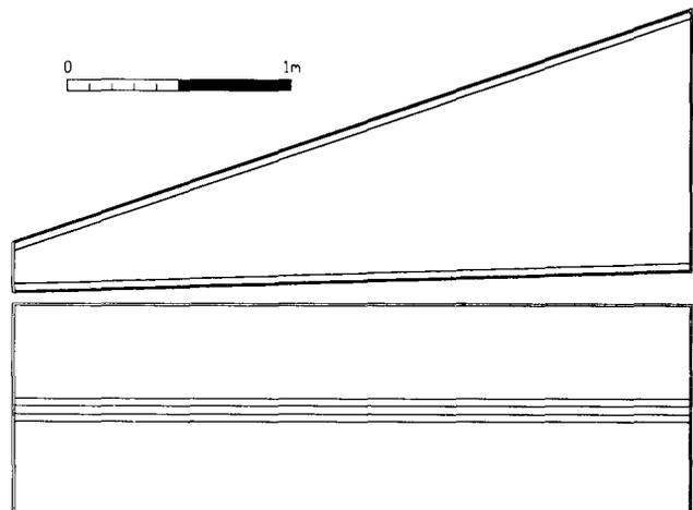
Figure 7: Top and side views of the horizontal half-wave resonator.
