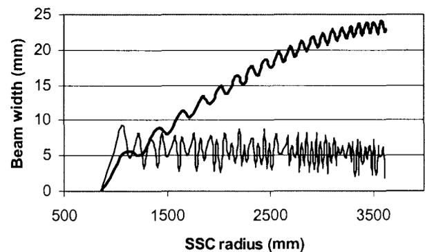
Figure 1: Beam width due to energy spread as a function of radius for a 20° long beam pulse without flat-topping (thick line) and for a 40° beam pulse with a flat-topping system, consisting of two dees in opposite valleys.
